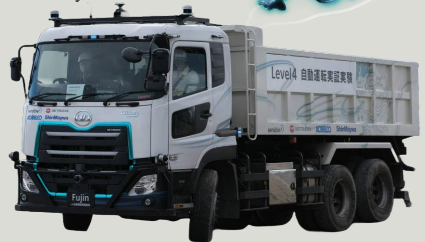
Level 4 autonomous demo truck 'Fujin'
